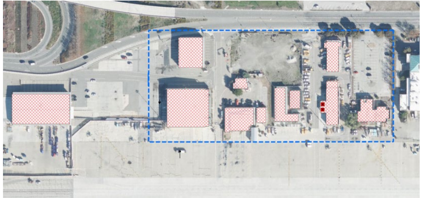
Preliminary site plan for construction of the New Belly Freight Facility and Receiving Center footprint and the associated buildings to be demolished
